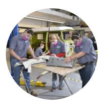
All teams were provided a pedal car kit and given the option of making modifications to the existing car or completely designing their own car. The only parts LISD TECH Center students used from the original Summit Racing pedal car were the frame, seat, pedals, and drive bars. Students stretched the original frame one foot and constructed a tubular roll cage. The steering and drive train were modified by LISD TECH Center Advanced Manufacturing students to fit the new frame. All
